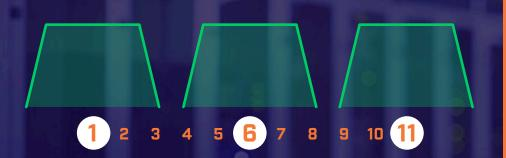
WiFi signal at 20 MHz has a very distinct shape. This shape leads to overlap on other WiFi channels that can be used for setting up Access Points. The channel is the WiFi frequency spectrum that it uses to communicate.
